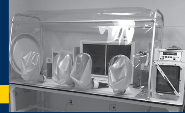
Rolf G. Freter, a professor of microbiology from 1966 to 1996, and engineer Dick Coy design the Coy Anaerobic Chamber to conduct studies on the anaerobic specimens that lived in the intestine of mice.
